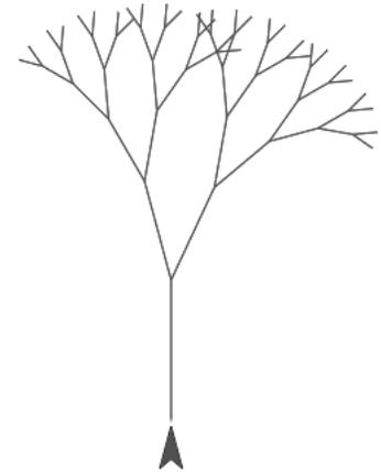
If recursion is new to you, here are a few brief hints: It's crucial that the recursion have a *base case*, that is, some small(est) case that the block can handle without using recursion. In this example, it's the case **depth=0**, for which the block does nothing at all, because of the enclosing **if**. Without a base case, the recursion would run forever, calling itself over and over.
